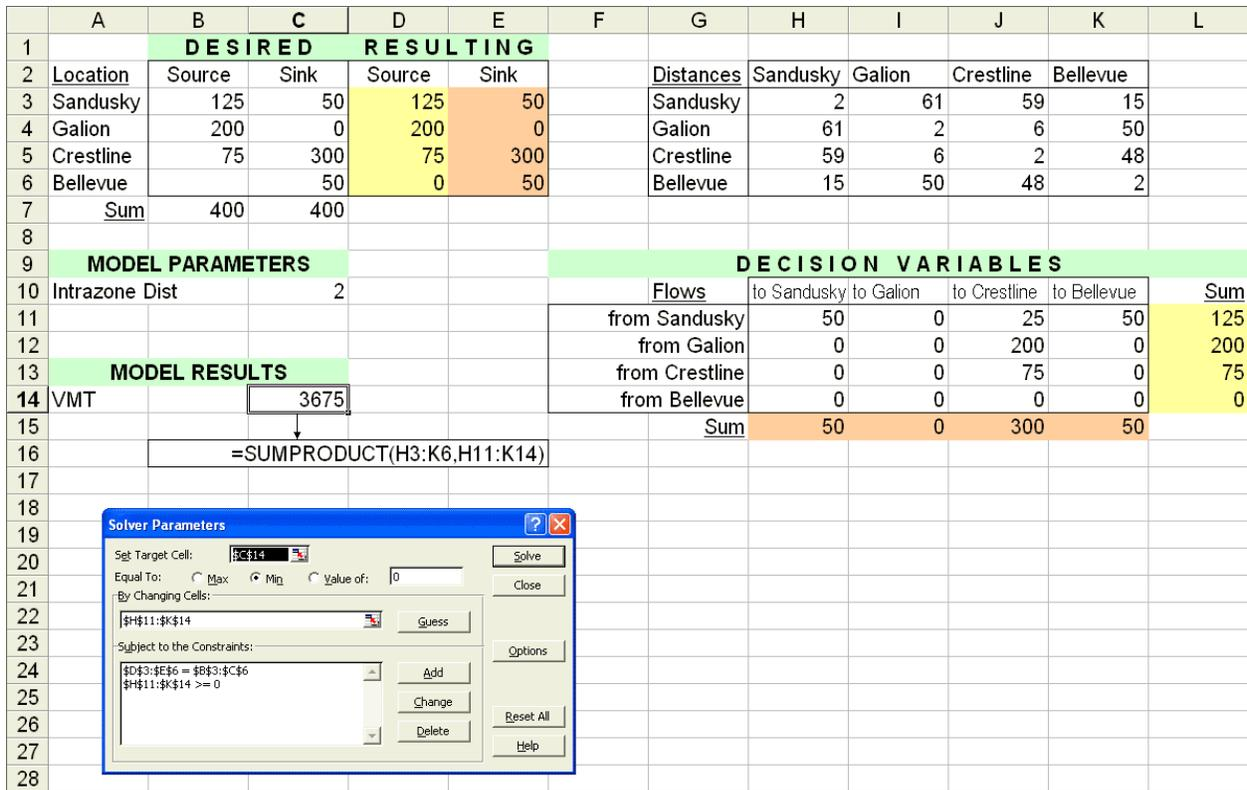
**Figure 2: Developing a mileage-minimizing model with Excel® Solver**
