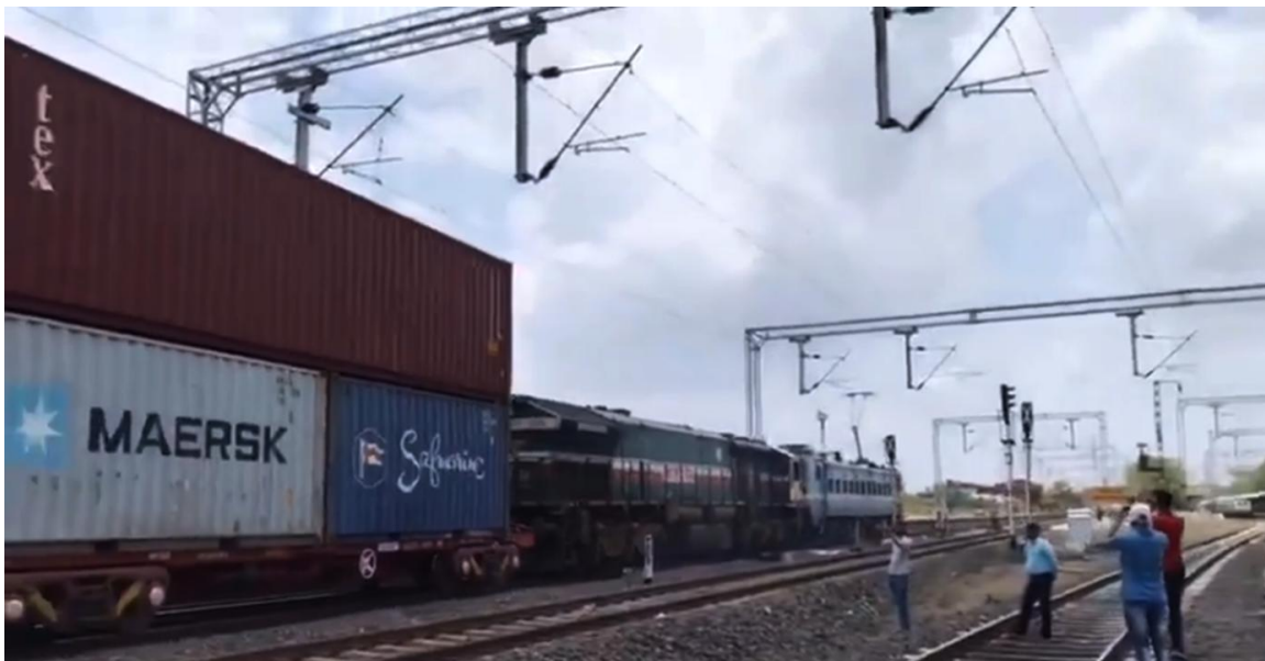
Figure 18. On Indian Railways, the Western Railway operates this electrified double-stack container train from Palanpur to Botad in Gujarat, June 10, 2020; Piyush Goyal photo (Government of India Open Data License via http://indianrailways.gov.in/ ).
